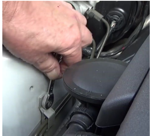
Release pipe clamp (allows booster to move)
